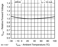
Fig. 3 - Relative Forward Voltage vs. Ambient Temperature
