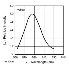
Fig. 6 - Relative Intensity vs. Wavelength
