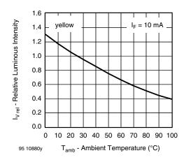
Fig. 5 - Relative Luminous Intensity vs. Ambient Temperature
