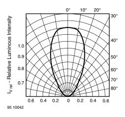
Fig. 7 - Relative Luminous Intensity vs. Angular Displacement
